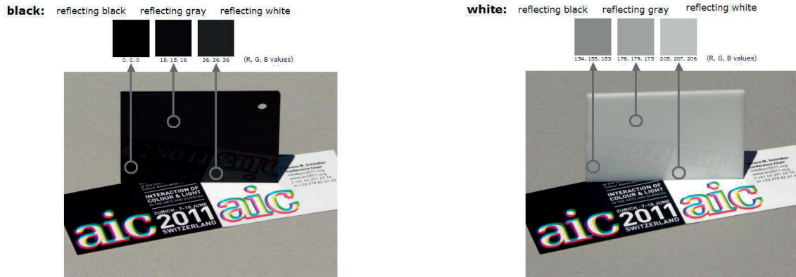
Figure 2. Black and white glossy surfaces reflect the AIC 2011 card (with black, white and chromatic colors) and the gray background. Above, the zones where black, gray and white are reflected in each case are extracted and measured.
