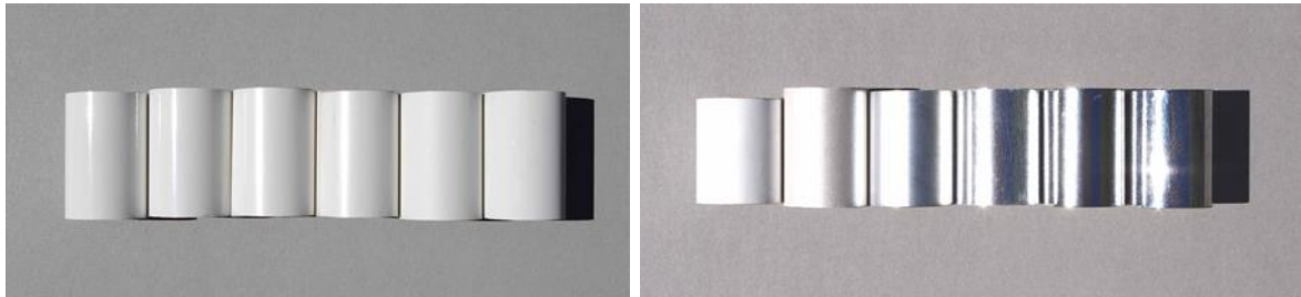
Figure 22: Two groups of cylinders from figure 20 showing scales of increasing gloss in one direction (left) and increasing metallic lustre in the other (right). The scales have matte white as a common starting point.
