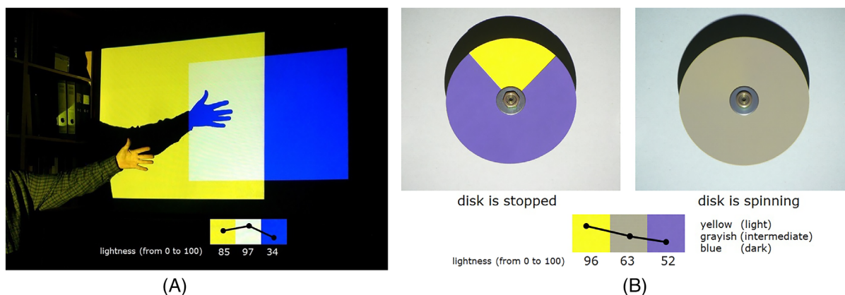
FIGURE 5 A, Overlapping lights produce an additive mixture: blue + yellow (red + green) = white; the resulting color is brighter. B, Spinning disks with color cardboards produce a partitive or optical mixture: blue + yellow = gray; the resulting color is an area-weighted average of both sectors' lightness: Yellow: 96% \times 0.25 = 24%. Blue: 52% \times 0.75 = 39%. The resulting grayish color is 24% + 39% = 63% L
